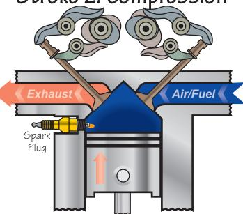
Spark occurs at the end of the stroke when the piston is "Top Dead Center", this is when the piston is at the highest point of its apex.
