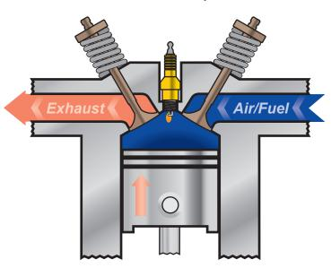
Spark occurs at the end of the stroke when the piston is "Top Dead Center", this is when the piston is at the highest point of its apex.
